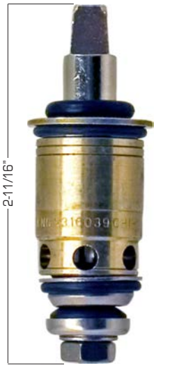
CHICAGO® 1-099XTJKABNF • 1-100XTJKABNF 1/4 Turn Hot (OEM) ▲131578 Cold (OEM) ▲131577 Hot ▲100421 Cold ▲100471 Packing 128335 O-Ring 128032 Faucet Washer Kit 128523 ▲101119
